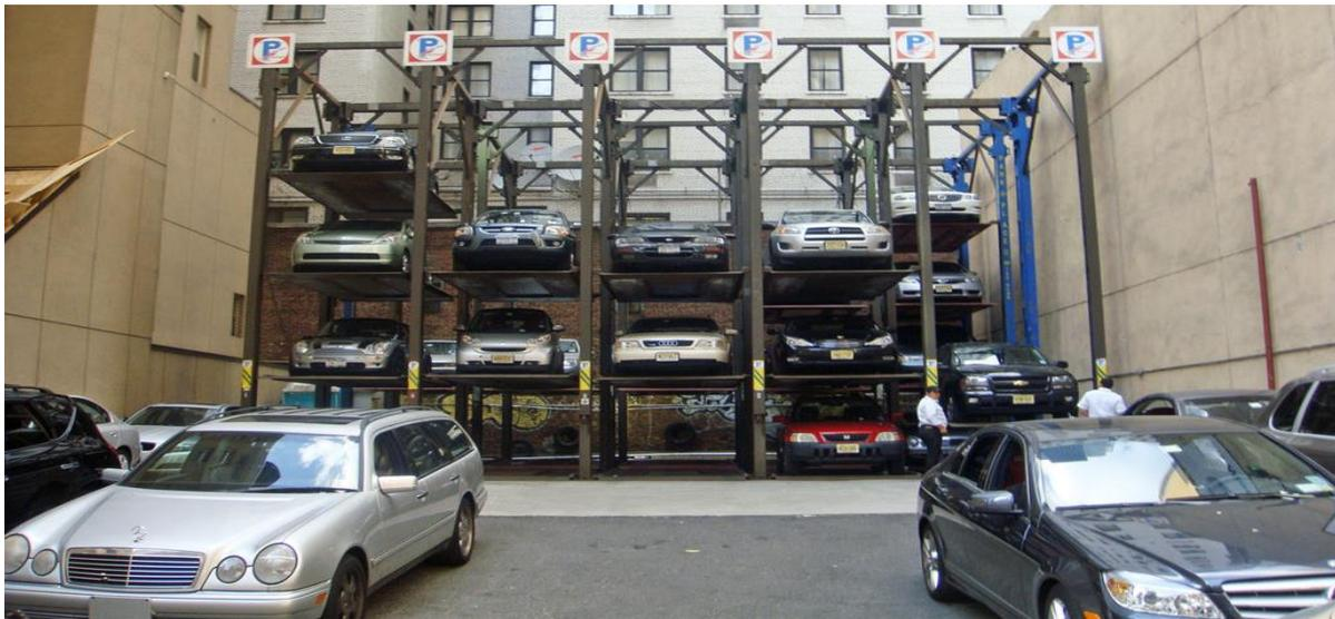
Figure 20 Multi-level stack parking NYC
