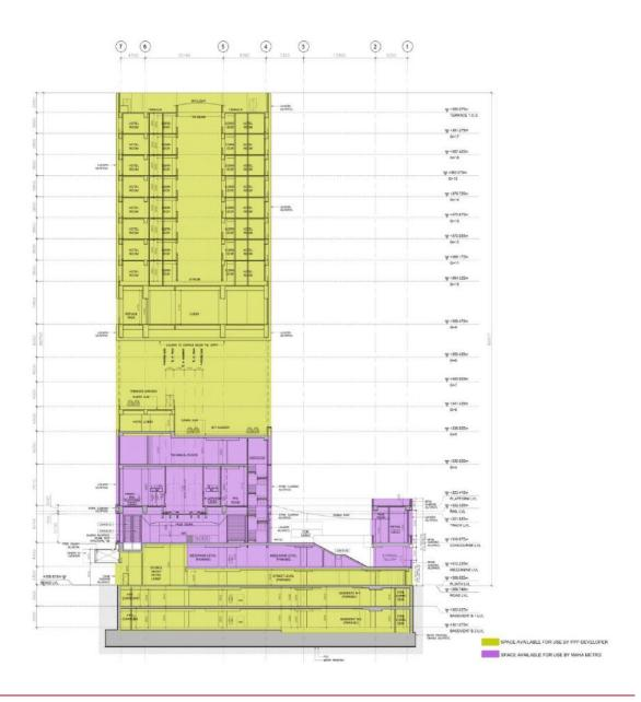
The configuration of the Zero Mile Station building and Proposed Property Development over airspace of Zero Mile Station building is as per table attached in Annexure. Attached drawings in Annexure defines the Architectural Controls of Proposed Property Development Building.
