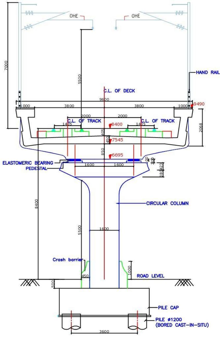
TYPICAL SECTION OF VIADUCT WITH U GIRDER
