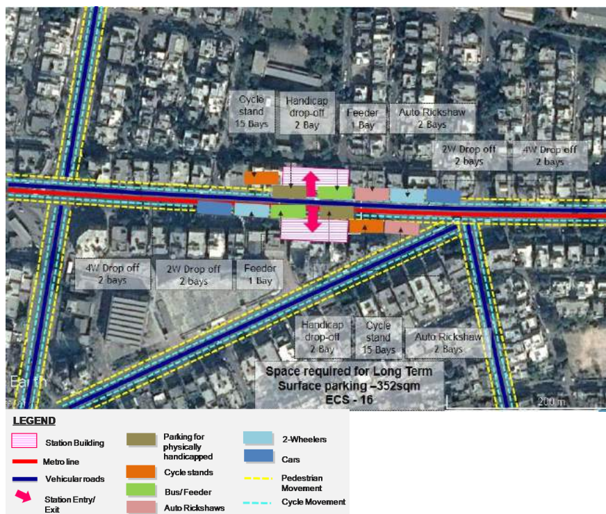
FIGURE A- 121 : CONCEPTUAL LOCATIONS FOR PICK AND DROP, PARKING AROUND VAISHNODEVI SQUARE STATION
