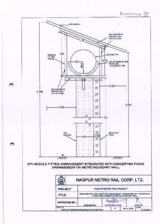
Conceptual array layout for mounting structure at track walls: The capacity and panel layout shown is only indicative and tentative. The successful bidder has to finalize the design as per the requirement, site availability and submit for approval of MAHA-METRO. The mounting structure is already installed on the track walls. Bidders are advised to visit the site for more details.
