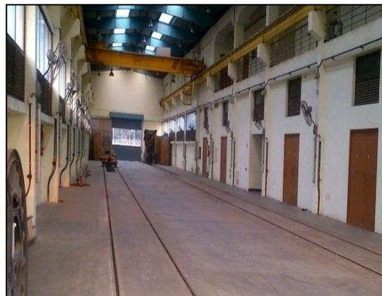
may be housed and given required inspection attention in a separate shed called ETU workshop, for which 1 line have been provided in the depots. However for the heavy lifting needs, these vehicles may be taken to main workshop for required attention.
